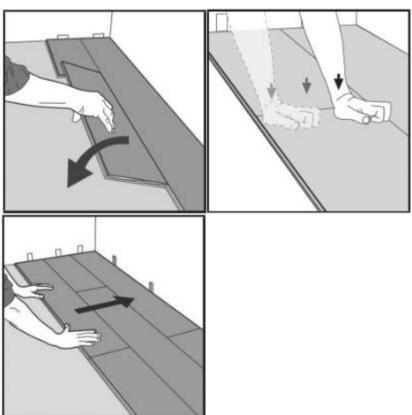
**<u>Disassembly Guide:</u>** Definitive Hybrid Flooring can be disassembled and reassembled if necessary as long as the flooring is not damaged. Disassemble the planks by sliding horizontally as shown in diagrams below.
